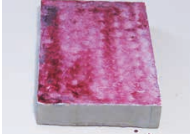
Prototype of a DysCrete solar cell, series of experiments with red dyes
