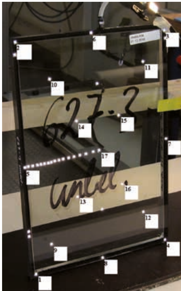
Test specimens prepared for an experiment on the deformation behaviour of multi-pane insulating glazing made of thin glass
