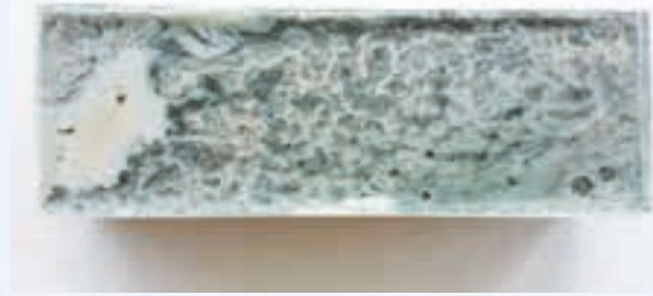
Prototype of a DysCrete solar cell, series of experiments with green dyes
