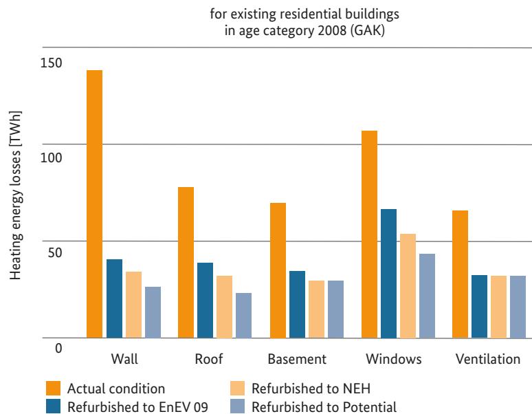
Figure 4: Total heating energy losses per building component in various states: unrefurbished (actual condition) or refurbished to standards of the Energy Saving Ordinance (EnEV 09), to the level of a typical low-energy house, or to Passivhaus standard (potential) for existing residential buildings in age category 2008 (GAK)
