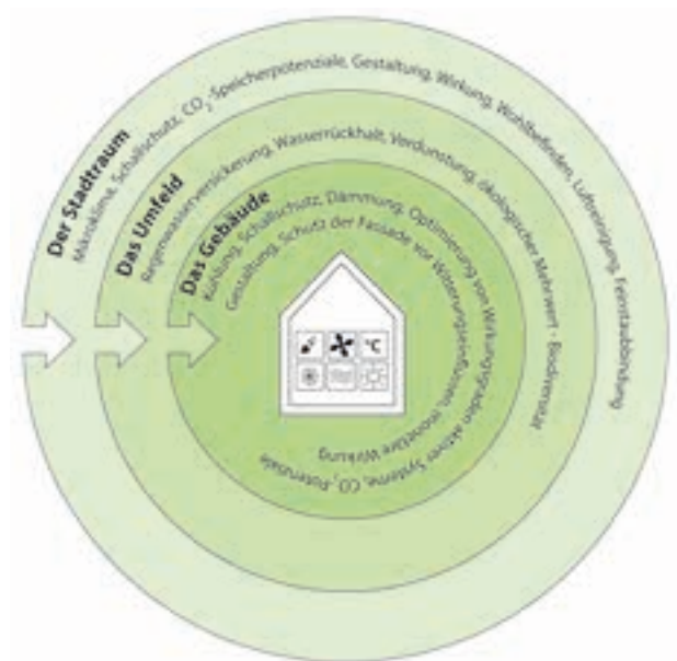
Figure 2: Measures to meet a building's demand for electricity, fresh air, and water in its day-to-day operation and life cycle aspects associated with manufacturing components; a depiction of synergies and competing aspects in a planted building
