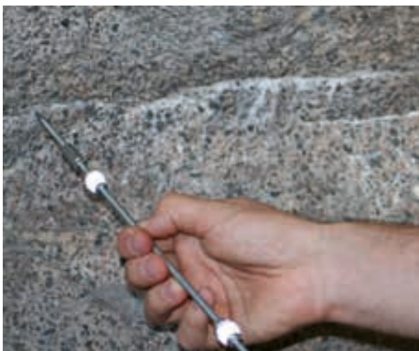
Figure 1a und 1b: Crack tracking system with scanning probe (a) and camera system (b)
