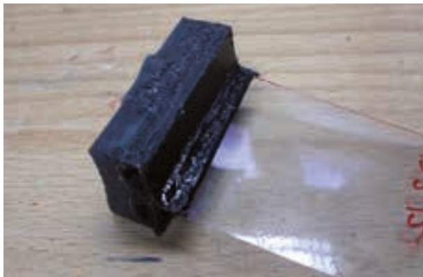
Test specimen with film in the cavity between the panes following a pull-out test; the film adheres to the secondary sealant on both sides.
