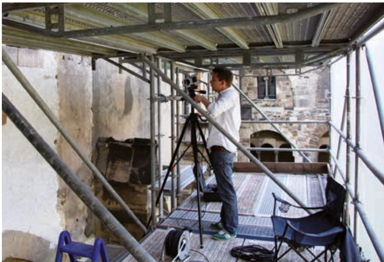
Figure 4a: Recording thermography sequences on the surface of the plaster in Magdeburg cathedral following artificial heating
