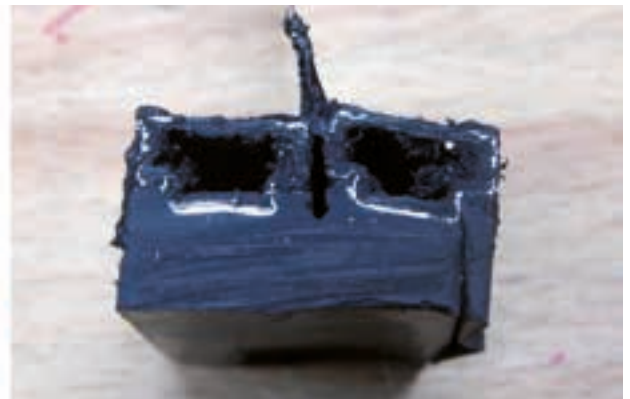
Test specimen with film in the cavity between the panes following a pull-out test; the film adheres to the secondary sealant on both sides.
